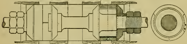
An Old and Successful Piston Valve.
